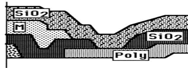
Faulty metal-poly contact
